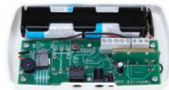
Fig 2 Valve Control: Battery position
